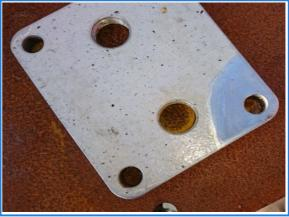
Part exposed to 3 months of open exposure to rainfall and saline environment. The jelly can be easily wiped off when required
